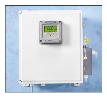
are 0-2 or 0-20 PPM, with a low end resolution of about 0.05 PPM. Response time to changes in ammonia concentration is less than 60 seconds to 90% of a step change in concentration, making the system much faster responding than competitive monitors. Two programmable alarm relays are available for local alarm functions, and two analog 4-20 mA output signals are provided for interface to plant DCS, telemetry, or other supervisory instrumentation.
